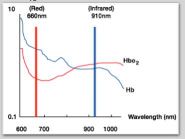
At 800nm (the isobestic point) the absorption coefficients are identical. The opposite side of the probe has a photocell that detects the amplitude of the red and infrared lights. The ratios of these amplitudes allows the microprocessor to give an estimate of the SpO2 by comparing the values with those from tables stored in its memory produced from experimental data.
